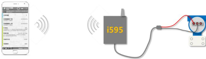
The i595 hardware is a WiFi to HART adapter, it can work as WiFi AP or Station mode. When adapter work in “local” mode, it work as a AP essentially, also, When adapter work in “remote” mode, it work as a station essentially.
