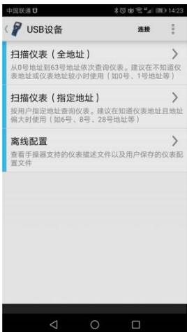
The screenshot shows the 'USB设备' (USB Device) connection menu. The title bar says 'USB设备' and '连接'. There are three main options listed: '扫描仪表 (全地址)' (Scan meters (all addresses)), '扫描仪表 (指定地址)' (Scan meters (specified address)), and '离线配置' (Offline configuration). Each option has a brief description and a right-pointing arrow. The '扫描仪表 (全地址)' option is highlighted with a blue bar on the left.                                                                                                |
